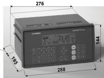
Front-of-panel-mounting unit VEG 20400 Front protected to IP 54, residual unit to IP 20, plastic Panel cut-out: 138.5 x 282 mm Weight: 3.5 kg
