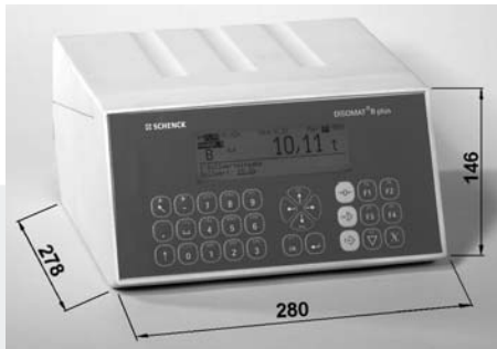
Desk-top housing VTG 20400 Protected to IP54, plastic 10 cable in let with power and load cell cables Weight: 3.7 kg
