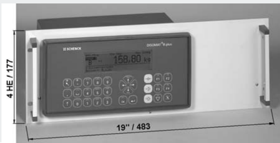
19“rack VNG 20400 With panel-mounting unit VEG 20400 Depth 195 mm for connecting cable Front protected to IP 54, residual unit to IP20 Weight: 7.5 kg
